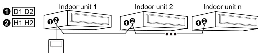
Fig.3.9.12 One wired controller controls multiple IDUs
