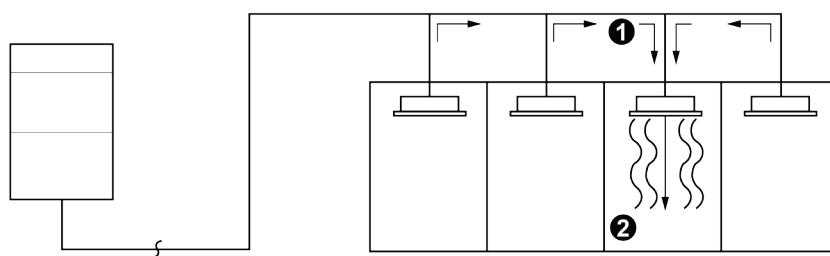
① Flow direction of refrigerant leakage
