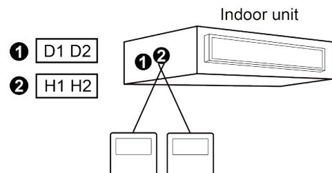
Fig.3.9.10 One wired controller controls one IDU    Fig.3.9.11 Two wired controllers control one IDU
